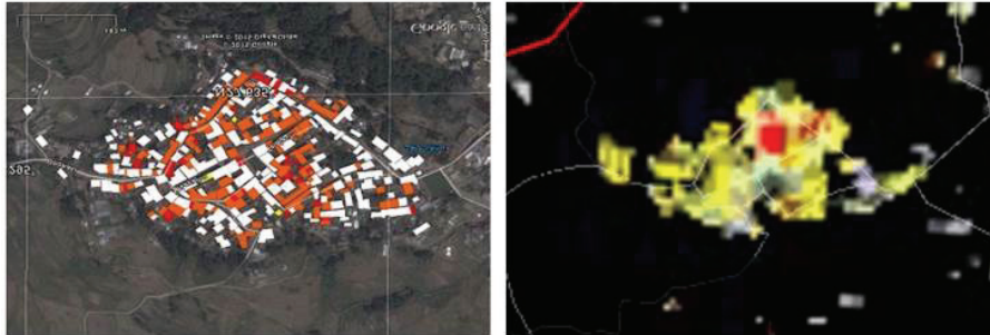
Figure 26 Coherence magnitude and the survey of damage extent for every house in Khokana.
