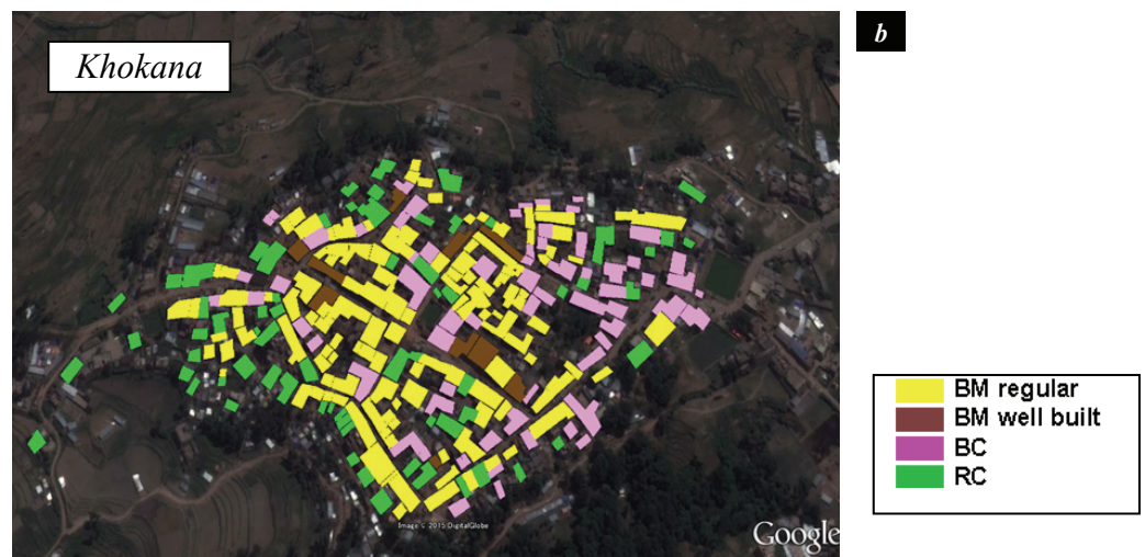
Figure 10 Survey of building type for every house in Sankhu and Khokana.
