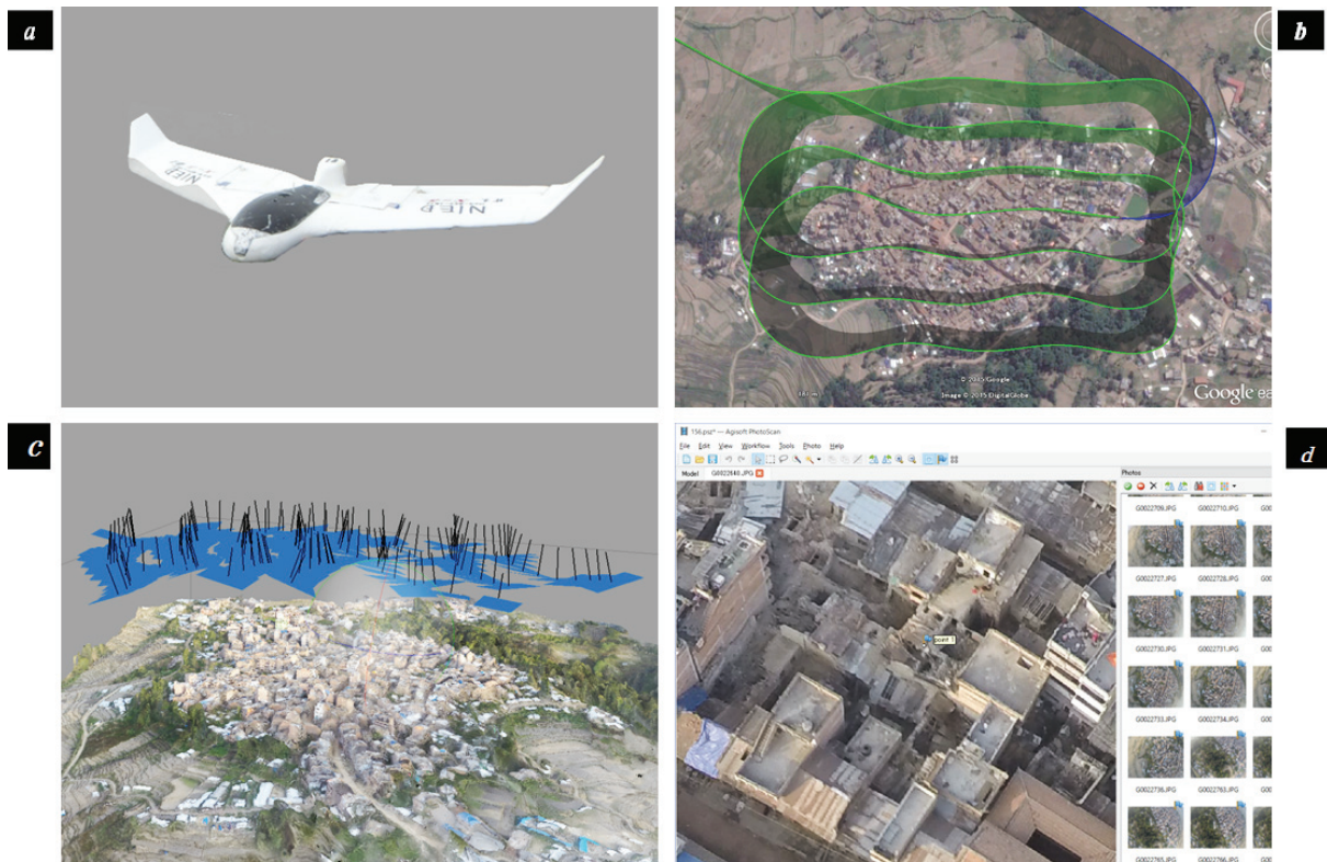
Figure 9 Building damage survey using compact UAV over Khokana.
