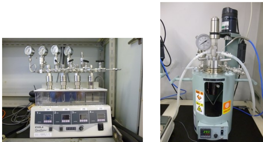
Fig.2-2. Reaction apparatus: 50 mL SUS316 stainless steel autoclave (left) and 100 mL Hastelloy autoclave (right).
