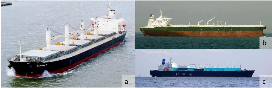
FIGURE 1.1: Several types of ships, (a)Bulk carrier ‘Sabrina I’, (b)Oil tanker ‘AbQaiq’, (c)LNG tanker ‘Puteri Firus Satu’.
