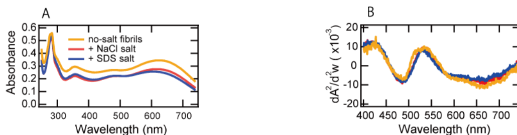
Figure 2-7. Effects of residual salts on iodine staining. (A) UV-vis absorption spectra of no-salt fibrils (orange) and no-salt fibrils containing NaCl (red) or SDS (blue) salts stained with iodine. (B) Second derivatives of the spectra in a range from 400 to 740 nm. Color codes are defined in the legends in the panel A, specifying types of fibrils.
