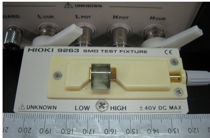
Fig. 2-2. The measuring chamber set on the test fixture 9263 that is attached to the impedance analyzer HIOKI IM3570.
