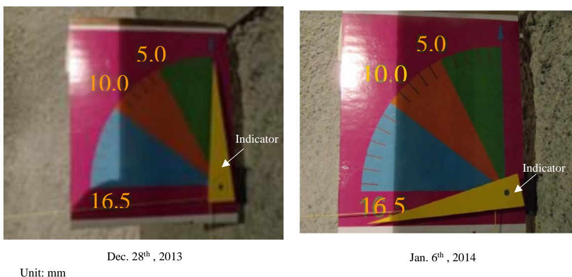
Figure 3.22 Rotation of the indicator visualizing change of the horizontal displacement
