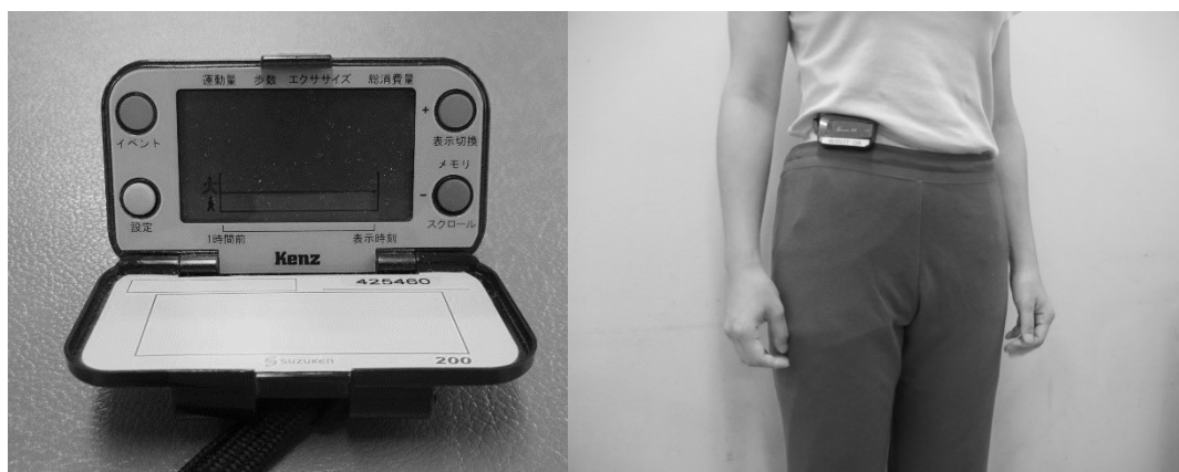
Figure 1. Device for measuring physical activity levels. Left: Lifecorder GS (Suzuken Corp., Nagoya, Japan). Right: A study participant wearing the accelerometer.
