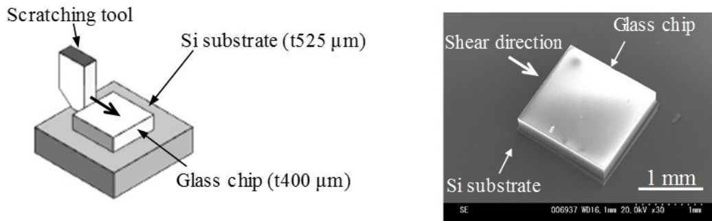
Figure 5.4. Schematic of shear strength test and SEM image of test specimen.
