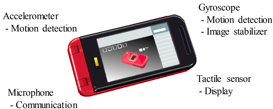
Figure 1.3 Schematic of MEMS sensors for smartphone.
