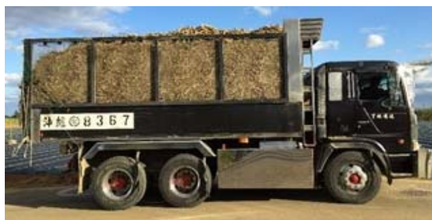
Figure 7.6 Truck used in the traffic loading test.
