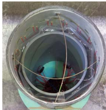
Figure 6.5 Airbags applying internal pressure.
