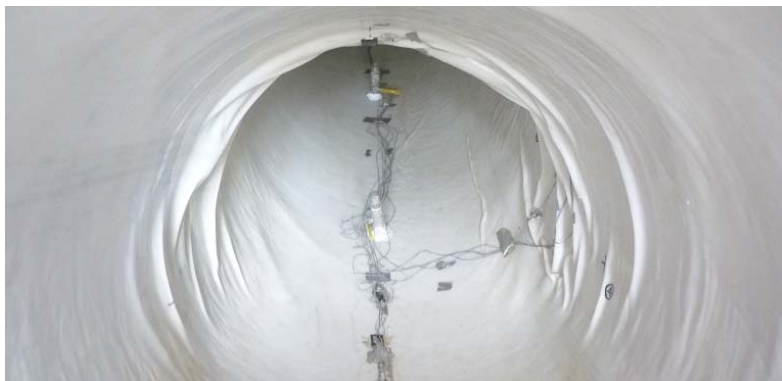
Figure 4.5 Wrinkles at the bend.
