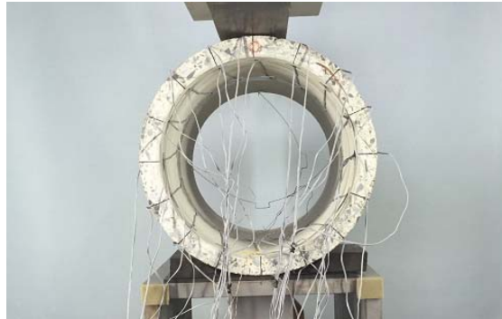
Figure 5.1 Parallel-plate loading test.
