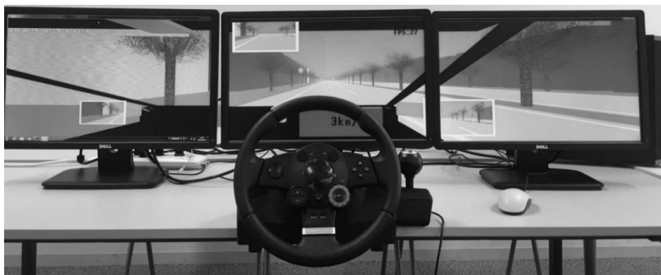
Figure 1. A depiction of the Driving Simulator
