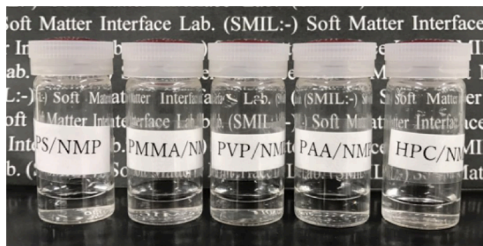
Figure 5. The dissolving ability of N-methyl pyrrolidone (NMP) to a various of polymer. To most polymers, such as polystyrene, poly methyl methacrylate and others, can be dissolved in NMP.
