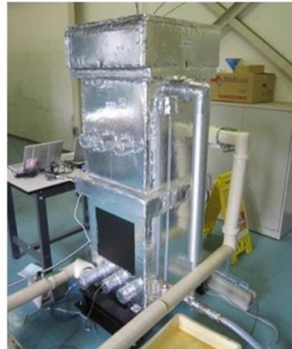
160 L heat storage tank
