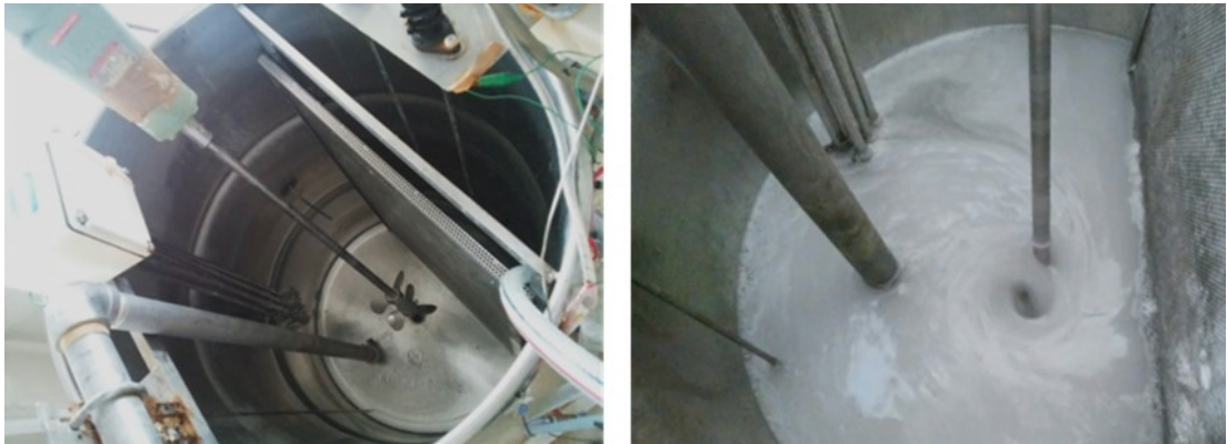
Fig. 3-6 Preparation of ammonia alum hydrate slurry in the tank
