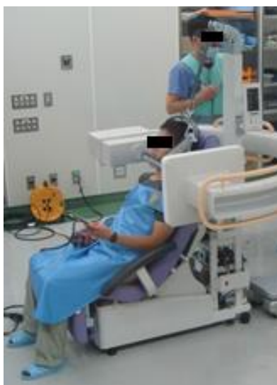
Figure 29. Cervical traction in inclined position during radiographic experiment.
