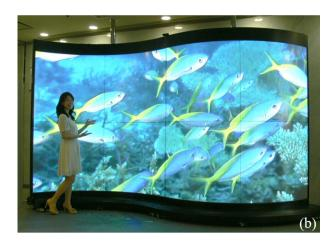
Figure 1.4: Photographs of super large-sized PDPs; (a) 145-inch 8K4K PDP [19] and (b) curved 180-inch PTA [20].
