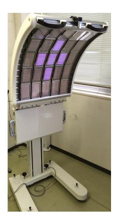
Figure 1.5: Photograph of a skin phototherapy system with UV LAFi emitting at 311 nm NB UVB [54].
