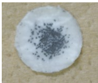
Figure 1-5. Lithium deposition on the glass separator at -5°C after cycle test in Fig.1-4.
