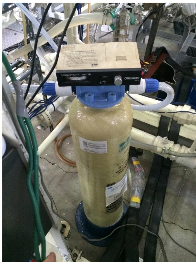
Fig 2.4 Ion exchanger
