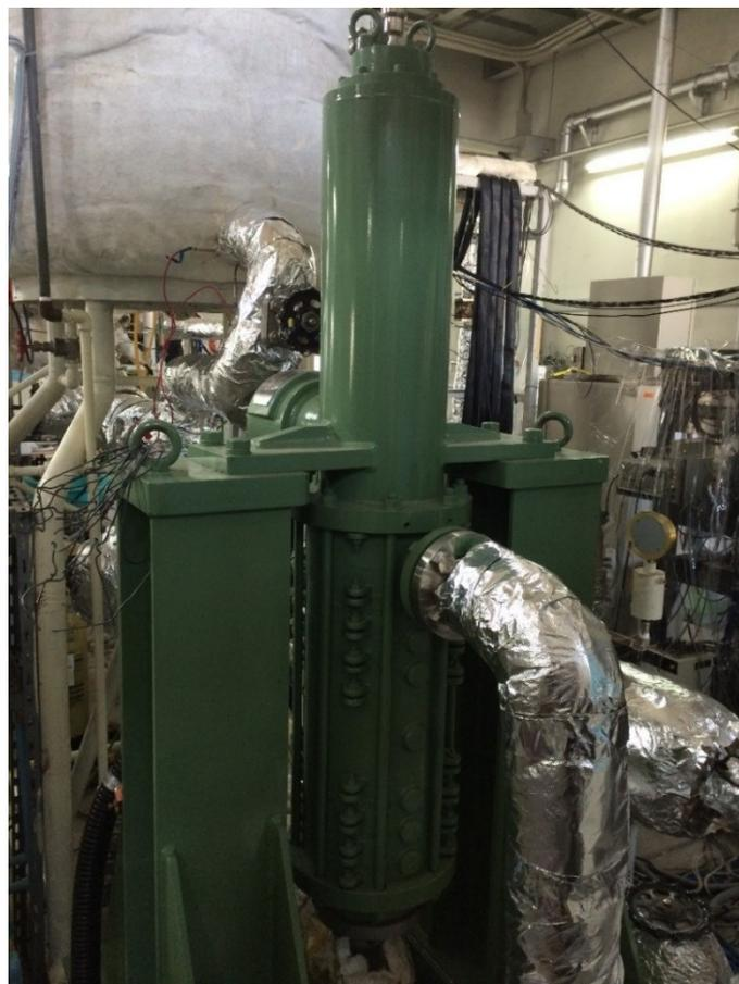
Fig 2.3 The canned-type circulation pump
