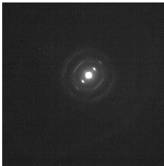
Fig. 4.59. Electron diffraction pattern of MWCNTs irradiated with \text{Ar}^{8+} at the fluence of 6 \times 10^{13} ions/cm 2 .
