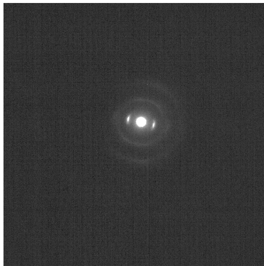
Fig. 4.61. Electron diffraction pattern of MWCNTs irradiated with \text{Ar}^{14+} at the fluence of 6 \times 10^{13} ions/cm 2 .
