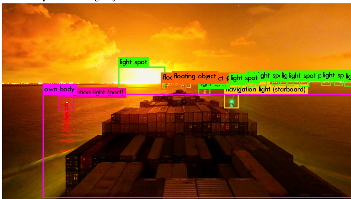
Fig.6.9 The recognition effect of the port and starboard lights
