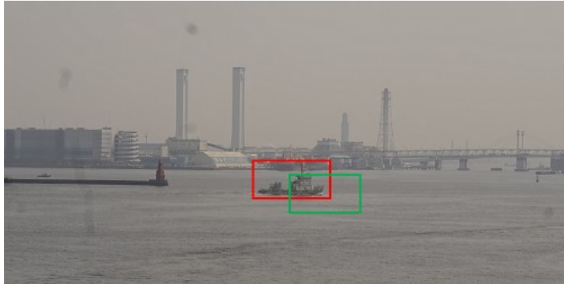
Fig.6.5 Example of intersection over union (IoU)
