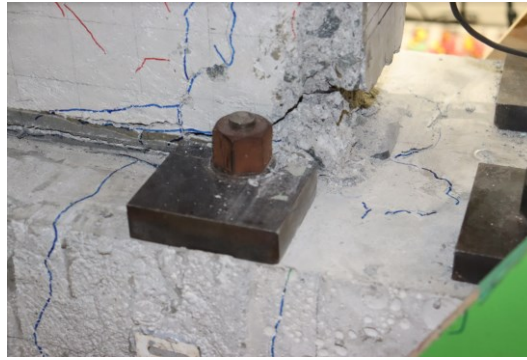
Fig. 4.3-6 Damage observed on specimen WP20-D10H55P-075
