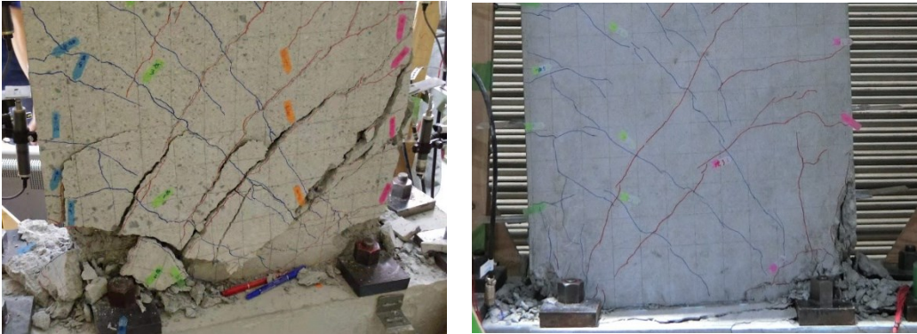
(a) W20-FU-15 (R=3%) (b) W20-HU-073 (R=3%) Fig. 2.3-7 Effect of the new arrangement method for D6 DL bars
