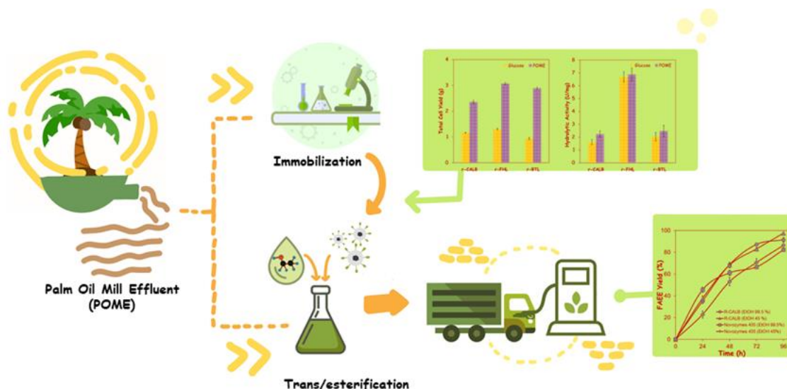
Fig. 1. Bioprocess concept of utilizing palm oil mill effluent (POME) for the immobilization of Aspergillus oryzae whole-cell lipase strains for biodiesel synthesis
