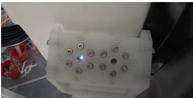
FIGURE 4.15. Installed laser head of the reflectivity monitor. The fibers are checked with a handy light source during the construction.
