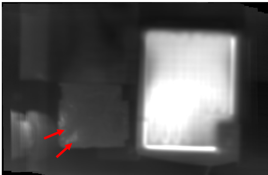
Fig.6-19 Result of reflection removal using monocular SfM
