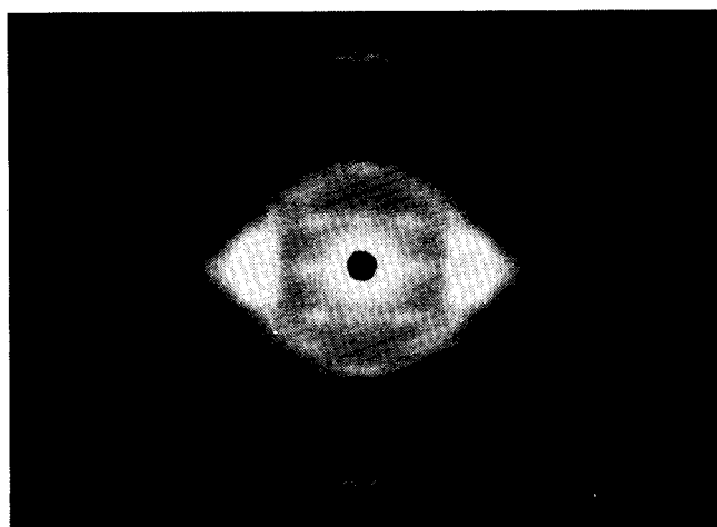
Fig. 1. X-ray fiber photograph of Nylon 6 \alpha -form at 22°C.
