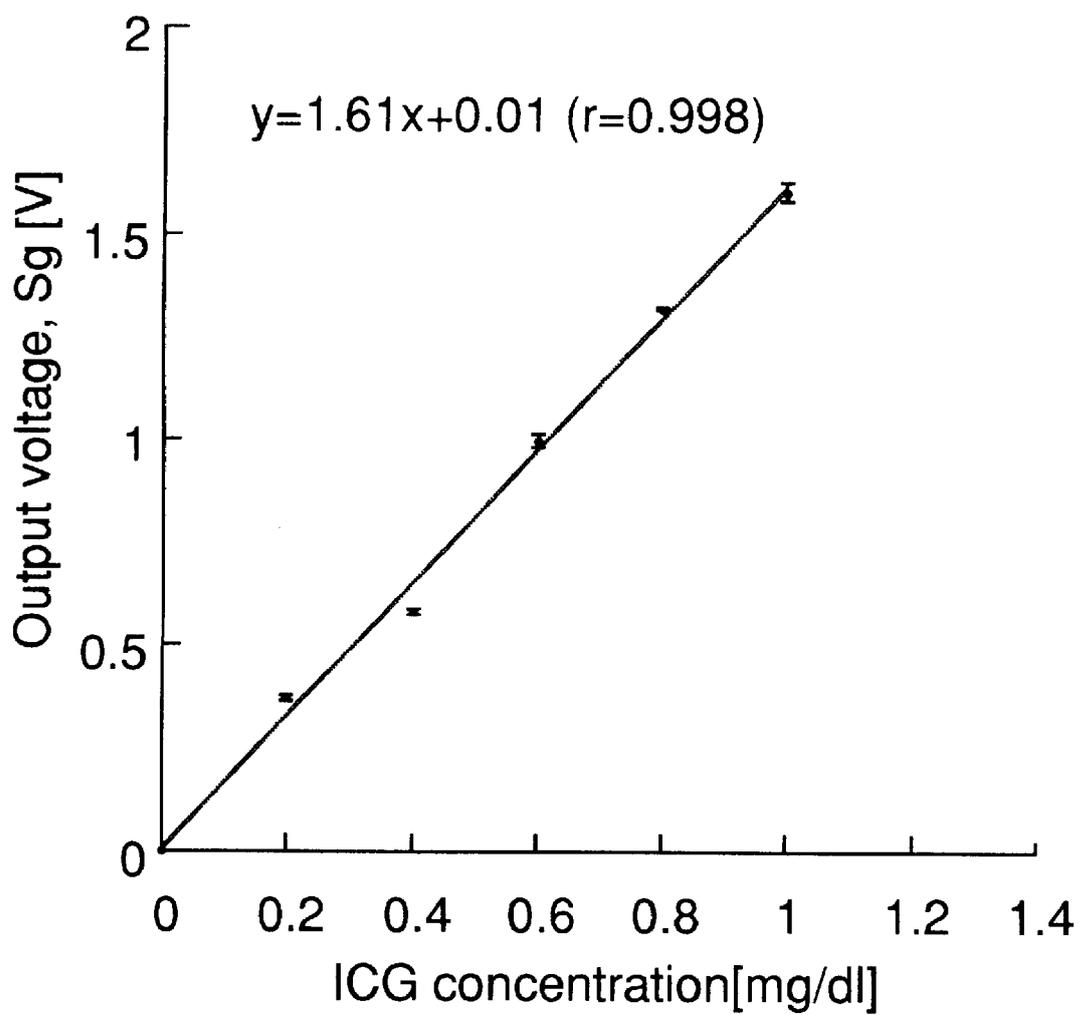
Figure 4.4 The linearity between ICG concentration and output voltage.
