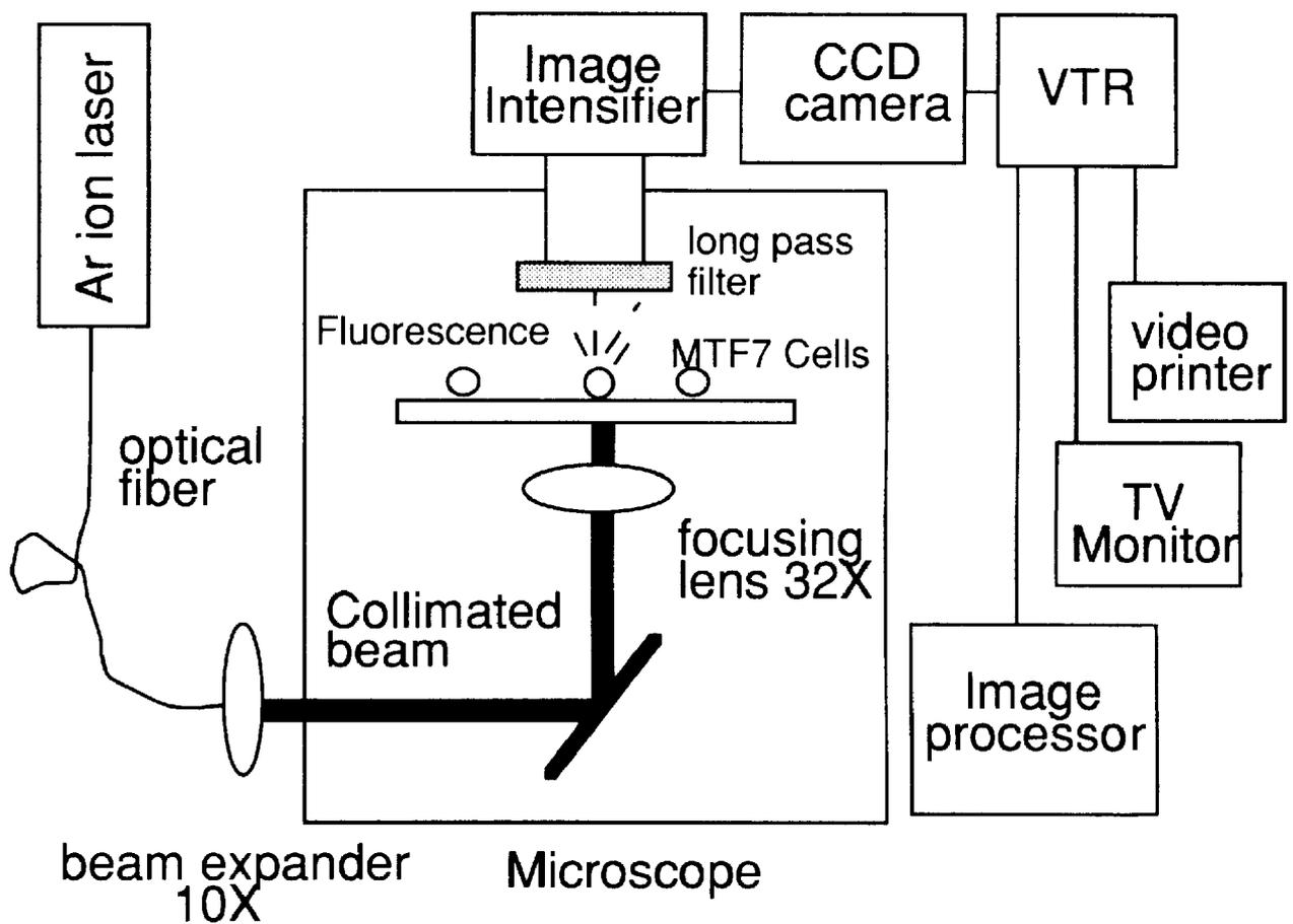
Figure 3.1: Fluorescence microscopy apparatus. An argon ion laser (488 nm) excited cellular PPIX fluorescence and an intensified CCD camera viewed the emission through a 580-nm long-pass filter.
