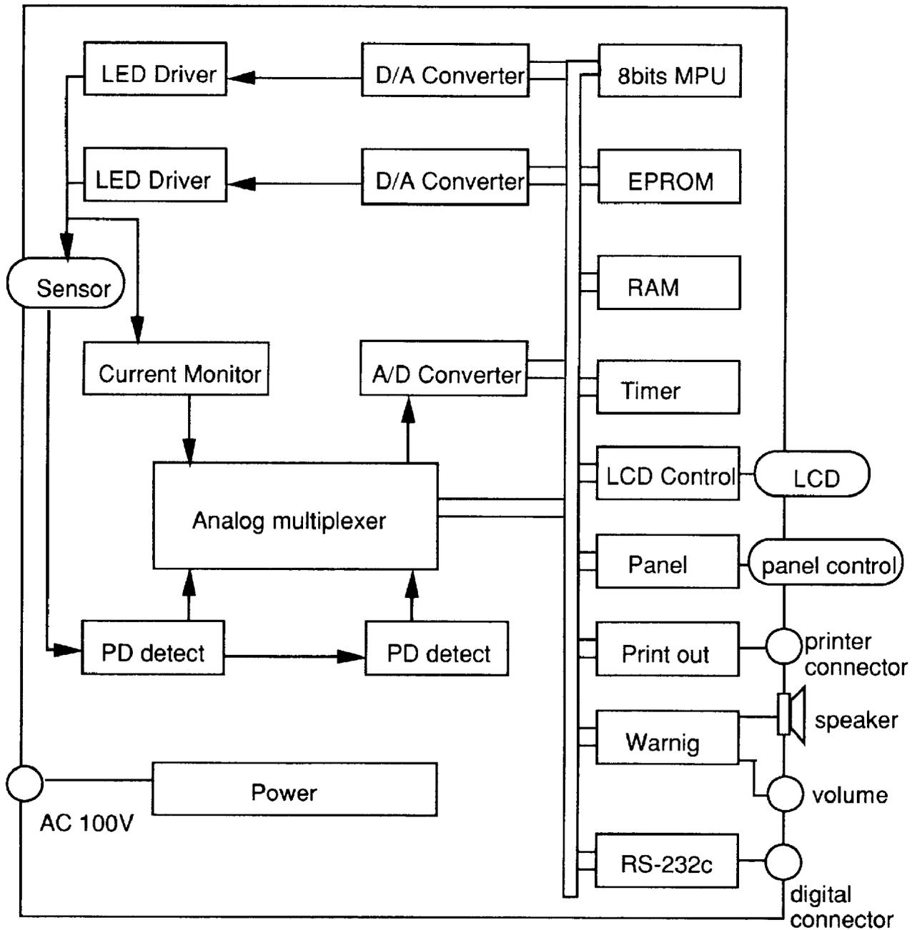
Figure 4. 3 Block diagram of the hardware system
