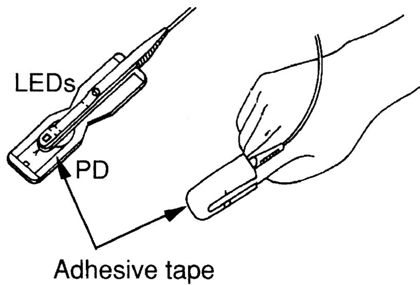
Figure 4.2: Optical Sensor attached to the fingertip
