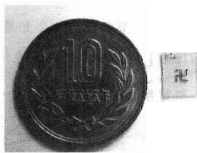
Fig. 5.5 Photograph of deposited metal “卍” shape structure using selectivity electroless plating method
