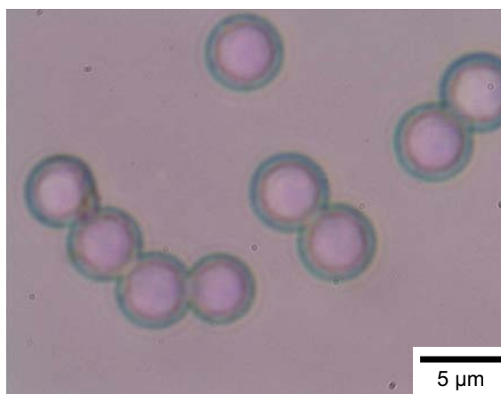
Fig. 2 An optical micrograph of PS/PDVB composite particles produced by seeded polymerization for the dispersion of (DVB/xylene)-swollen PS particles prepared utilizing the dynamic swelling method under the conditions listed in Table 2
