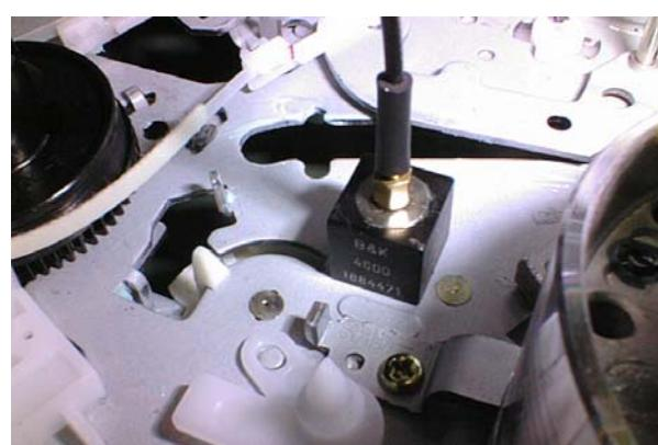
(c) The accelerometer set near the gear.
