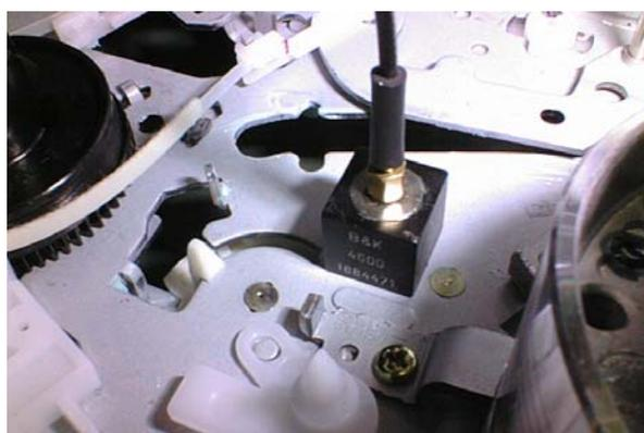
(c) The accelerometer set near the gear.
